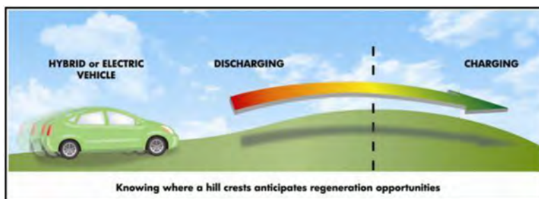
Figure 12. Road slope allows electric and hybrid electric vehicles to anticipate regeneration zones
