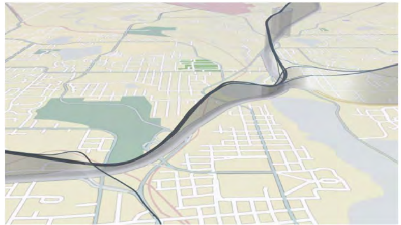
Figure 10. Road slope data is a key component of Predictive Cruise Control
