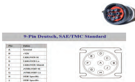
Figure 12 – J1939-13 Diagnostics Connector
