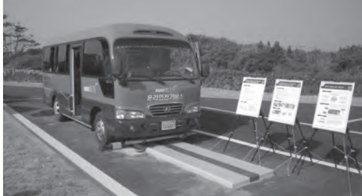
Fig. 10 A photo from the test bed with wireless charging facility
