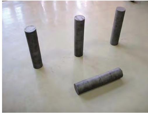
FIGURE 3 - Magnetic Markers (ferrite magnets with dimension: 25x100 mm).
