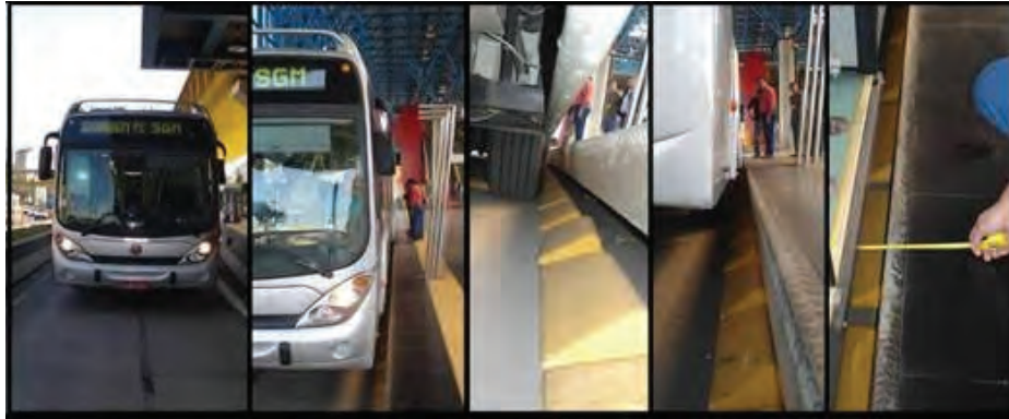
FIGURE 2 - Pictures sequence showing details of precision docking at bus stop platform. (Sao Paulo City's BRT, Mercado Station - Expresso Tiradentes).
