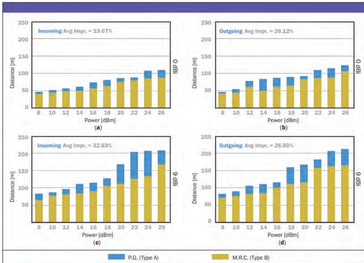
Figure 8. Test 1 and Test 2 (antenna diversity) communication range for the PSR of 70% and higher. The bottom two graphs are the results of the testing using 9 dBi antennas and the top two graphs are the results of the testing using 0 dBi antennas. The left two graphs are results of the incoming direction of the transmitter and right graphs are results of outgoing direction.
