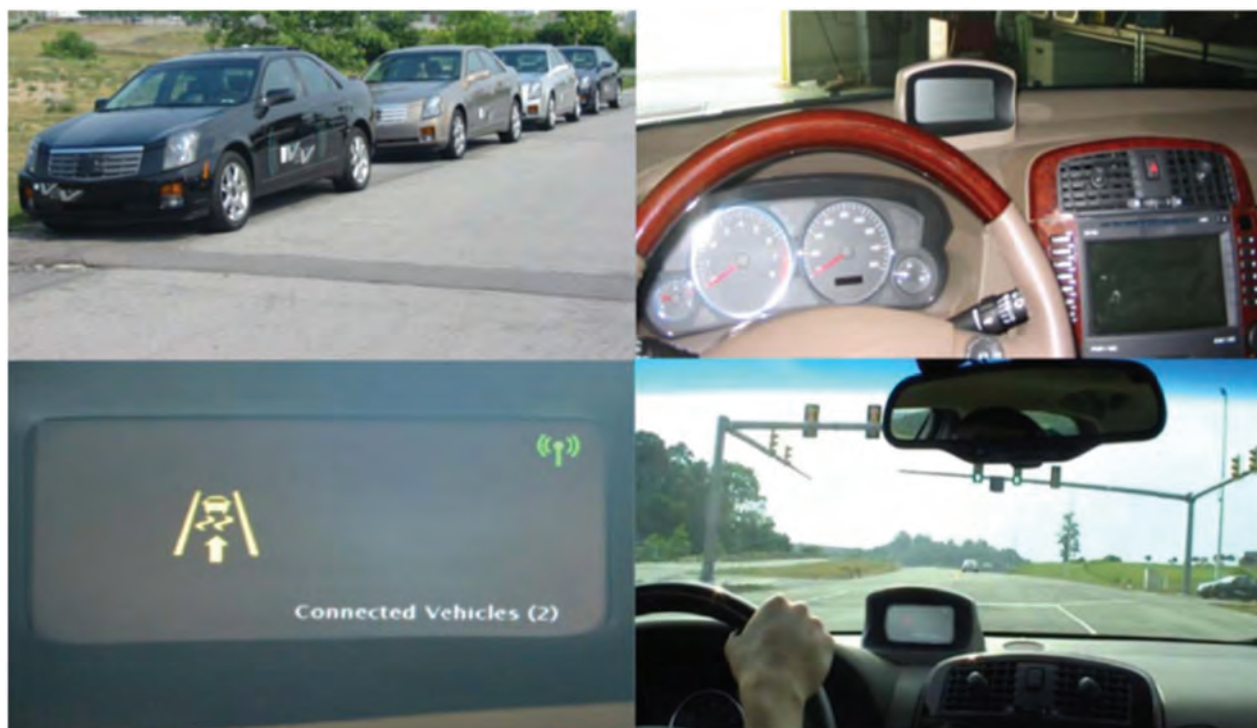
Figure 1. V2V Vehicles and DVI display mounted above the center stack
