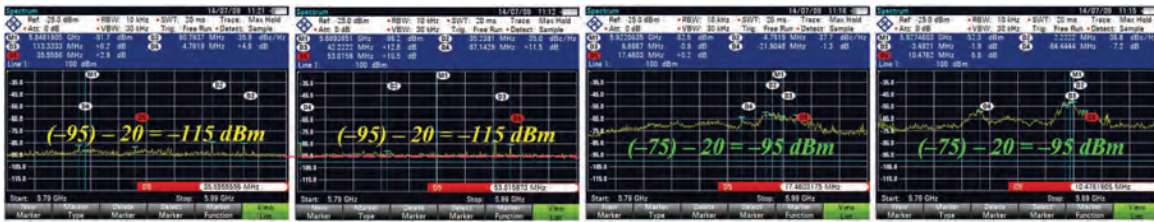
Figure 10. Background measurement using frequency spectrum.
