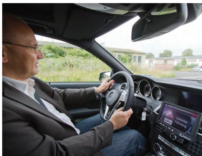
A car fitted with V2X wireless communications will receive early warnings of nearby V2X vehicles that become disabled.
