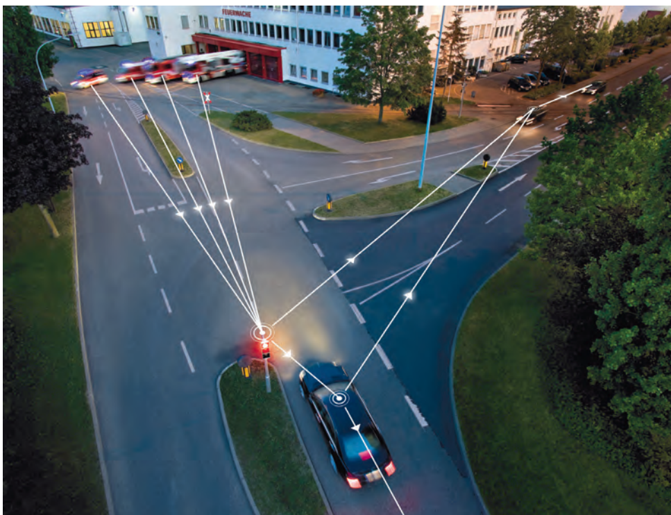
The simTD field test near Frankfurt, Germany, will evaluate rapid local data transfer among vehicles and roadway infrastructure.
