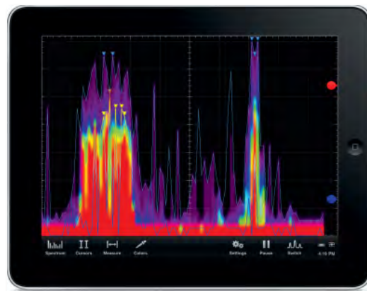
Figure 26: Spectral Analyses of 2.4GHz Band
