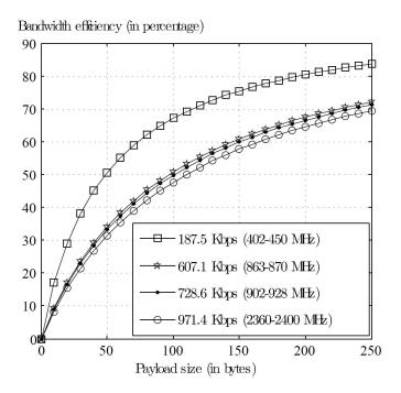
Fig. 8. Bandwidth efficiency of IEEE 802.15.6
