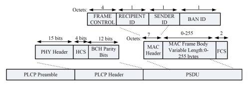
Fig. 3. IEEE 802.15.6 NB PPDU structure
