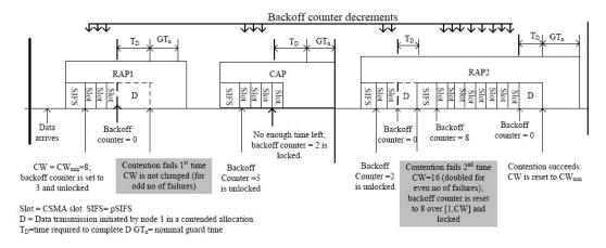
Fig. 7. CSMA/CA procedure in IEEE 802.15.6 standard
