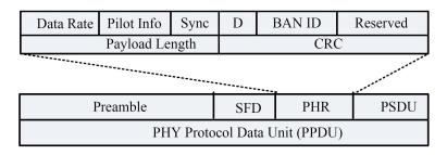
Fig. 5. IEEE 802.15.6 EFC PPDU structure
