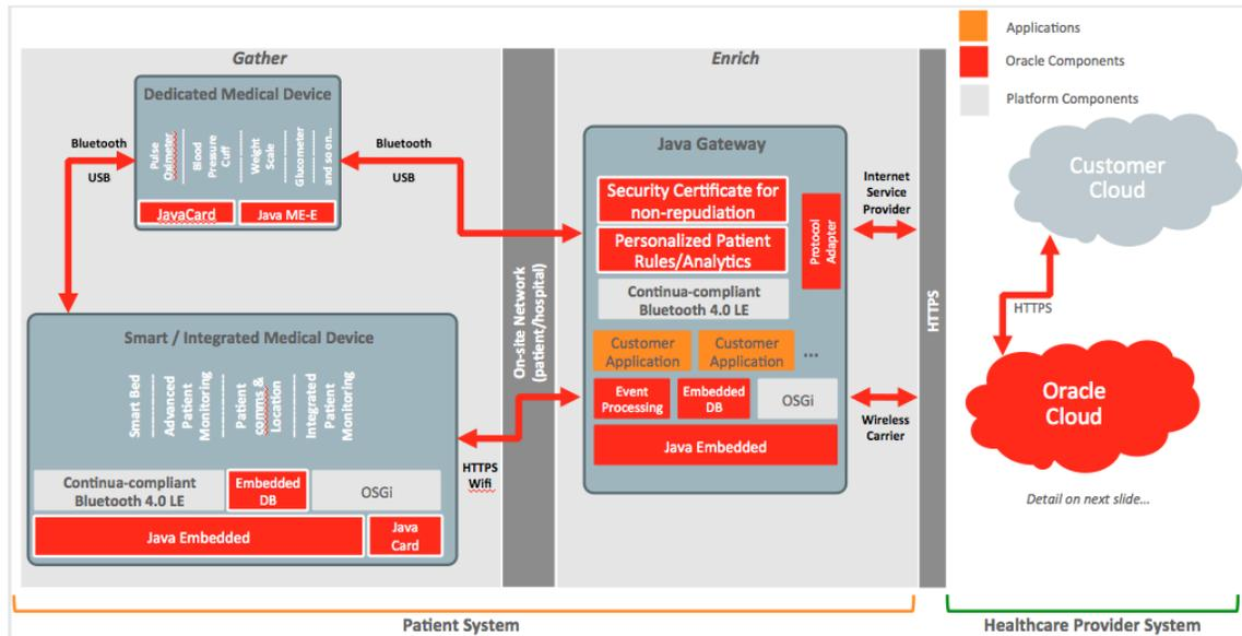
Figure 5. Oracle Java reference architecture for mHealth remote patient monitoring
