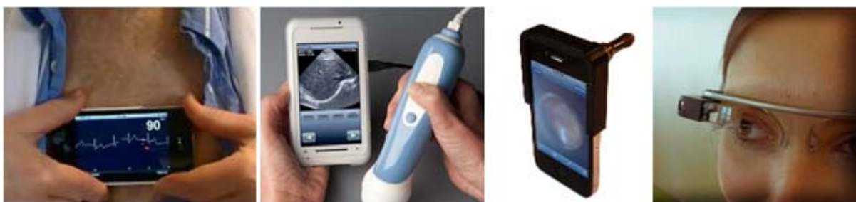
Figure 8. Internet of Things (IOT) Smartphone Peripherals and Next-Generation Wearable Computing: Consumer ECG, Mobile Ultrasound, CellScope, and Google's Project Glass (per Antonio Zugaldia).
